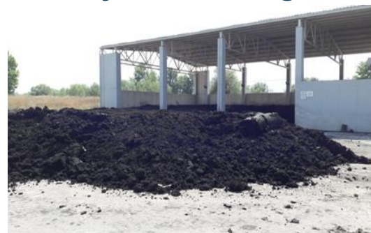
Temporary storage of dehydrated sludge
