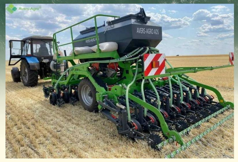
Precision direct seeder with a fertilizer tank that allows fertilization simultaneously with sowing
