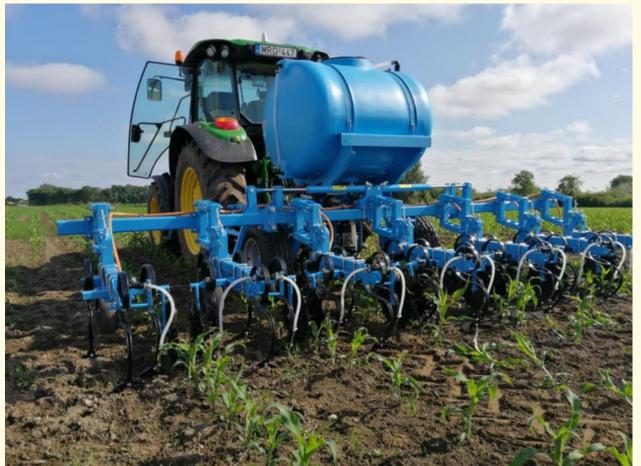
Cultivator with integrated liquid fertilization system, which allows localized application of fertilizers during operation, reducing nutrient losses and the number of passes over the soil
