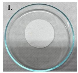
Glass fibre filter: pore size 0.7 µm
