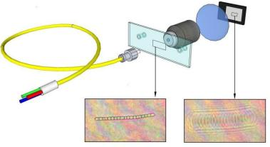
Holograms converted digitally into pictures giving intime and real time data on plankton taxa because of flow through chamber
