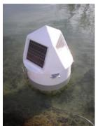
Buoy can be used digital and analog sensors, ion selective electrode UV and fluorescence probe.
