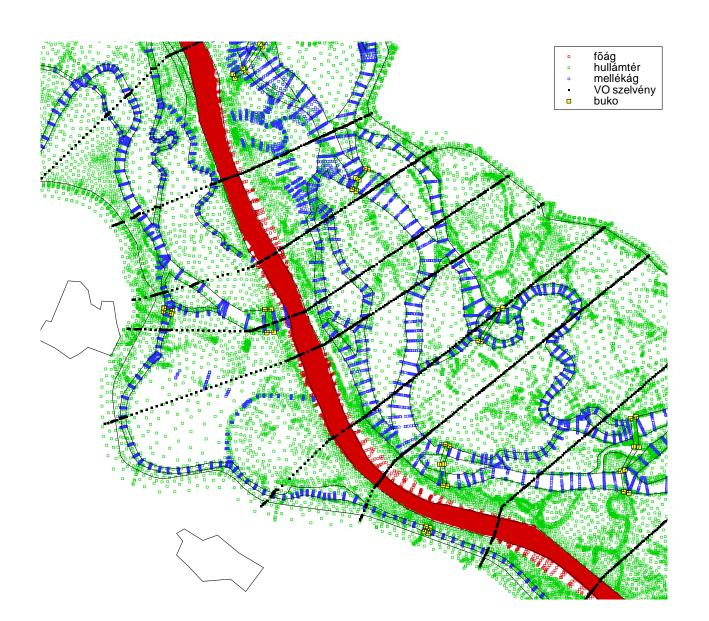
Past 2D flow modelling to help to understand the flood behaviour in the system
