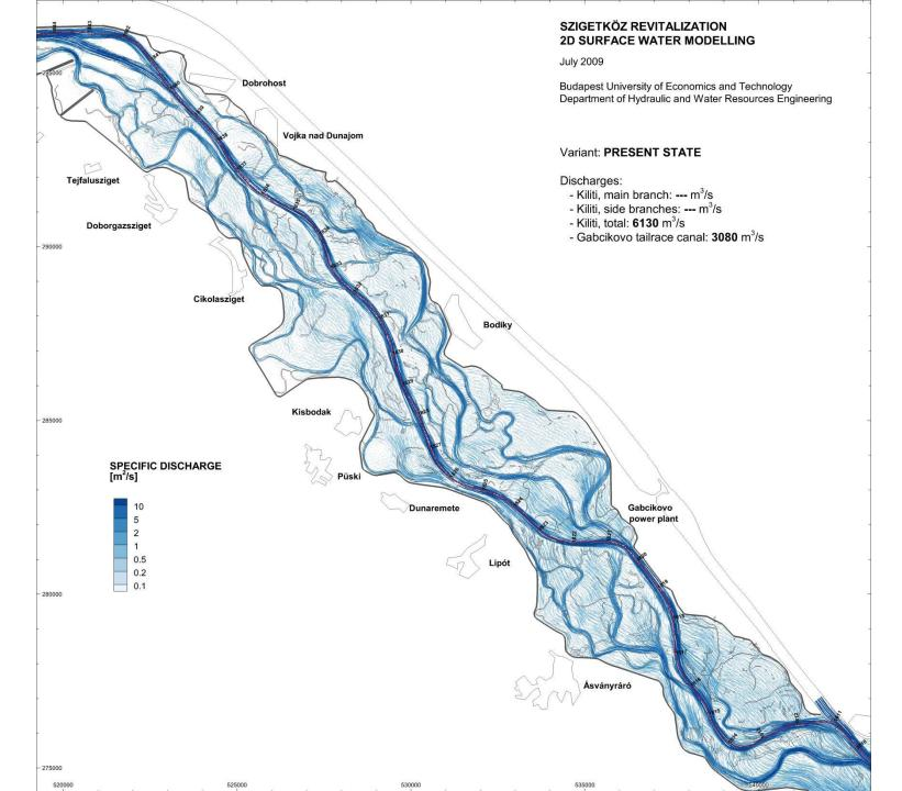
Detailed plan to capture the conveyance capacity distribution at the peaking
