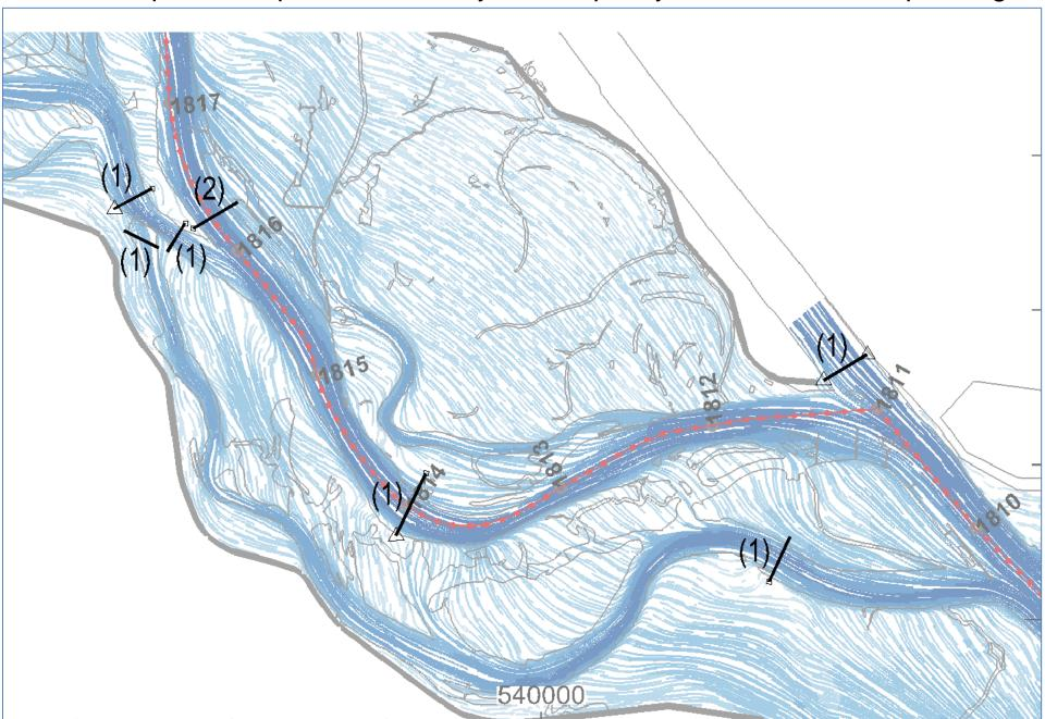
Detailed plan to capture the conveyance capacity distribution at the peaking
