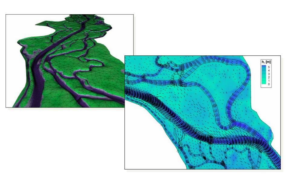
Past 2D flow modelling to help to understand the flood behaviour in the system
